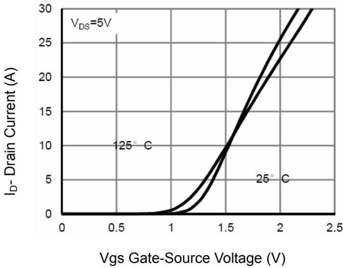
Figure 7 Transfer Characteristics
