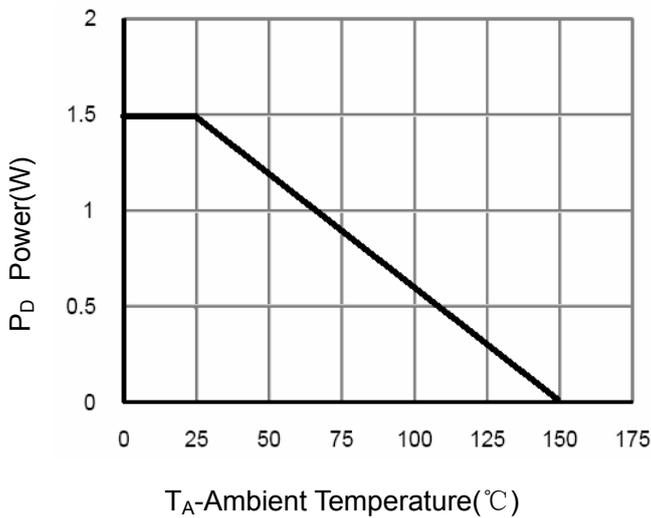
Figure 3 Power Dissipation
