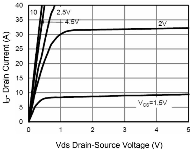
Figure 5 Output Characteristics
