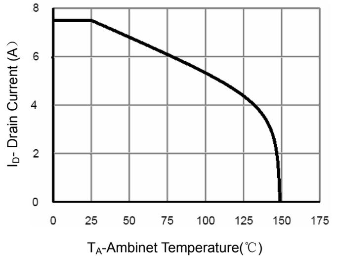
Figure 4 Drain Current
