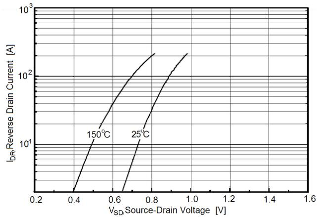
Figure4. Output Characteristics
