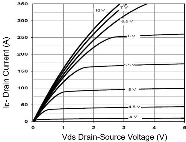
Figure 1 Output Characteristics
