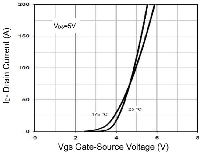
Figure 2 Transfer Characteristics
